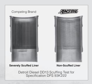
Based on third-party testing in the Detroit Diesel DD13 Scuffing Test for specification DFS 93K222.
