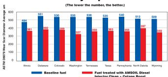
The ASTM D975 diesel fuel standard specifies a wear scar below 520  $\mu m$  in ASTM D6079 testing, while the Engine Manufacturers Association (EMA) specifies a wear scar below 460  $\mu m$ . Testing reveals AMSOIL Diesel Injector Clean + Cetane Boost provides significant lubricity improvement in diesel fuels found across the U.S., delivering improved wear protection. Fuels tested in 2017.
